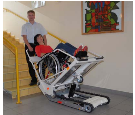
A powerful hydraulic piston adjusts the wheelchair platform position for travel on the stairs
